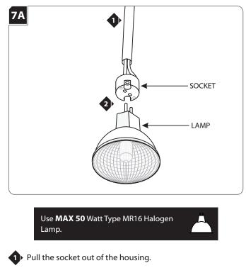
2 Push the lamp pins completely into the socket holes.
