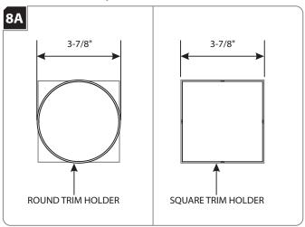
1 For round trims, mark a 3-7/8" diameter circle on drywall. Cut out the marked section. For square trims, mark a 3-7/8" square on drywall. Cut out the marked section.
