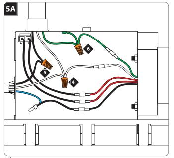
Connect the neutral power line wire to the white transformer wire and the white thermal protector wire with the wire nut.
