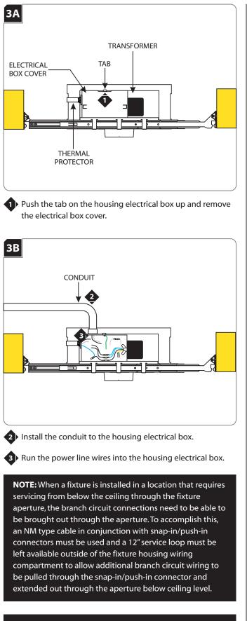
**WARNING:** <u>RISK OF FIRE</u>: When using the housing electrical box for power feed through, use <u>MAX</u> 4 - #12 AWG, or 6 - #14 AWG branch circuit wires.
