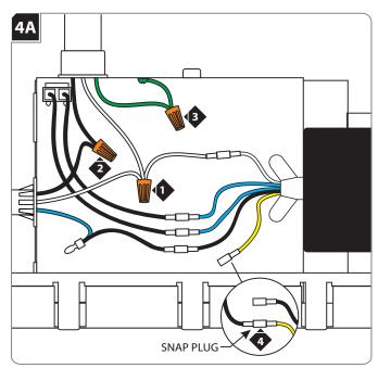
Connect the neutral power line wire to the white transformer wire and the white thermal protector with a wire nut.
