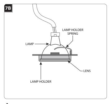
3 Ensure that the glass lens is properly inside the lamp holder.
