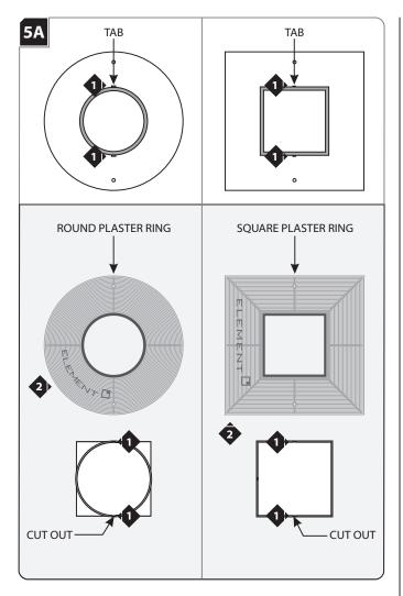
Line up the two tabs in back of the plaster ring with the two cut out sections of the trim holder inside edge.
