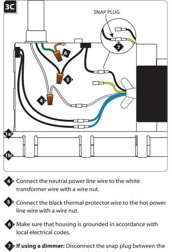
black transformer wire and the black thermal protector wire. Connect the yellow transformer wire snap plug to the black thermal protector wire snap plug. <u>If necessary</u>, <u>make sure to cap the black transformer wire snap plug</u>.
