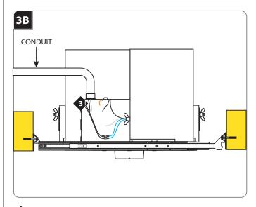
Install the conduit to the housing electrical box.
