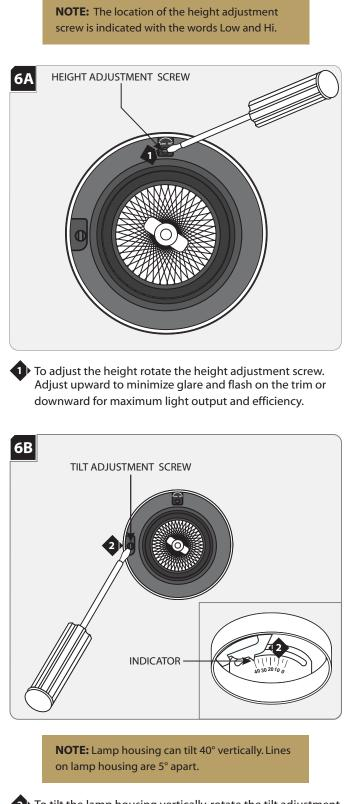
2 To tilt the lamp housing vertically, rotate the tilt adjustment screw until the desired angle is reached.
