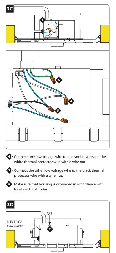
7 Replace the electrical box cover. Make sure that the top edge of the cover snaps under the tab.
