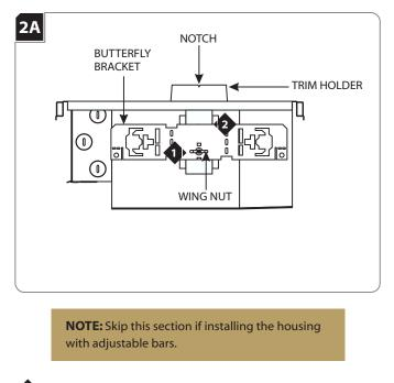
Slightly loosen the wing nut to slide the butterfly bracket up or down.
