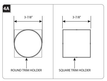
For round trims, mark a 3-7/8" diameter circle on drywall. Cut out the marked section. For square trims, mark a 3-7/8" square on drywall. Cut out the marked section.
