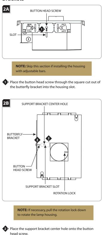
Push the support bracket slots against the butterfly bracket tabs.
