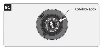
**NOTE:** Lamp housing can rotate 361° horizontally.
