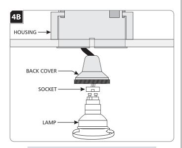
Use <u>ONLY</u> 120 Volt, **20** Watt GX10 Base MR16 Ceramic Metal Halide lamp with model numbers E3\_-C20AN.
