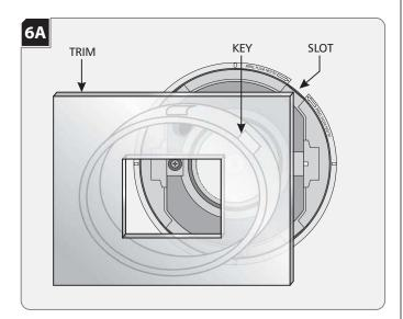
Line up the trim key with the slot in the housing and push the trim into the housing.
