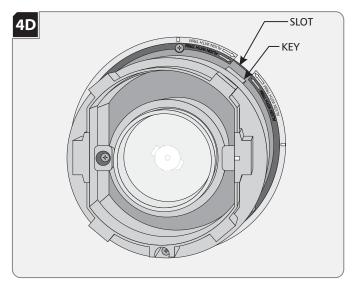
Line up the lamp holder key with the slot in the housing and push the lamp holder in to the housing until the magnets take hold.
