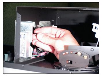
Remove the two thumb nuts inside the electrical box. These thumb nuts hold the ballast in place.
