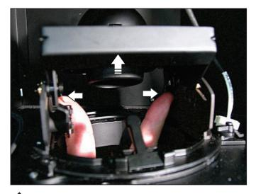
Squeeze the tabs to release the lamp housing and push the housing back.
