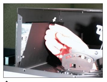
Pull the handle on the access door and remove the door.
