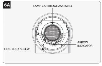
**NOTE:** Lamp cartridge assembly can rotate 180° horizontally. Lines on lamp housing are 5° apart.
