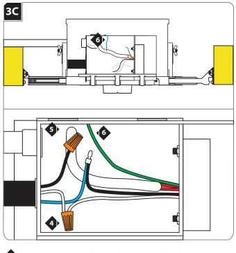
4 Connect the neutral power line wire to the white transformer wire and the white thermal protector wire with a wire nut.
