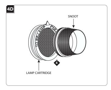
4 Replace and tighten the snoot completely to the lamp cartridge.
