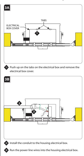
**WARNING:** <u>RISK OF FIRE:</u> When using the housing electrical box for power feed through, use <u>MAX</u> 4 - #12 AWG, or 6 - #14 AWG branch circuit wires.
