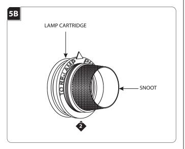
Unscrew the snoot from the lamp cartridge.
