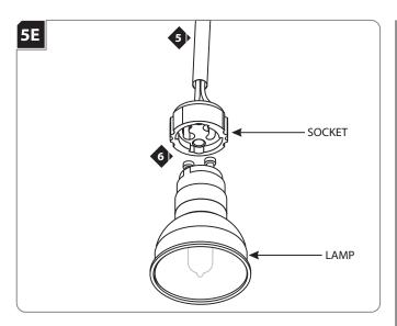
Use ONLY 120 Volt, 20 Watt GX10 Base MR16 Ceramic Metal Halide lamp with models E3RLB-C20DC\_, E3RLF-C20DC\_, E3SLB-C20DC\_.
