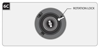
**NOTE:** Lamp housing can rotate 361° horizontally.
