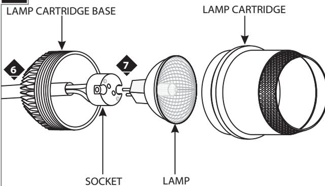
Use **MAX 50 Watt** Type MR16 Halogen Lamp.
