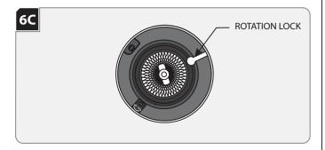
**NOTE:** Lamp housing can rotate 361° horizontally.
