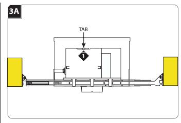
Push up on the tabs on the electrical box and remove the electrical box cover.
