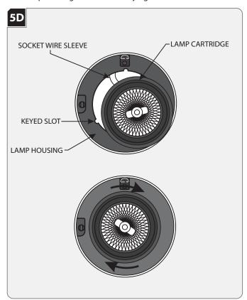
Feed the socket wire sleeve back into the lamp housing and align the lamp assembly with the keyed slots on the lamp housing.
