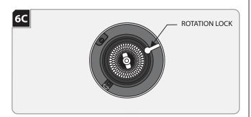
**NOTE:** Lamp housing can rotate 361° horizontally.
