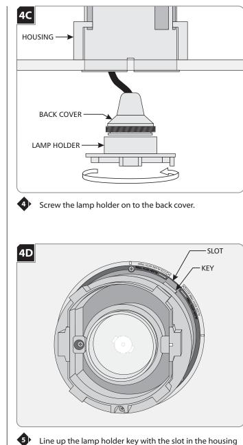
Line up the lamp holder key with the slot in the housing and push the lamp holder in to the housing until the magnets take hold.
