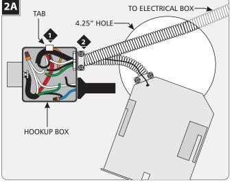
Lift the spring tab and remove the cover from the hookup box.
