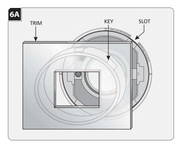
Line up the trim key with the slot in the housing and push the trim into the housing.
