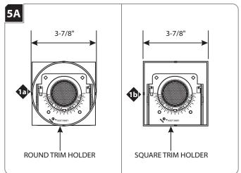
For housings with round trim holder, mark a 3-7/8" diameter circle on drywall. Cut out the marked section.
