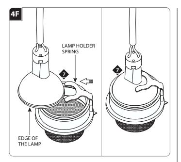
**7** Slide the lamp holder spring completely onto back of the MR16 lamp so that the edge of the lamp snaps into the lamp cartridge assembly.
