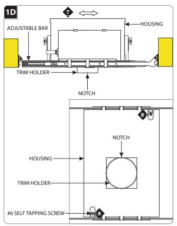
Adjust the trim holder position (horizontal position) by sliding the housing on adjustable bars.
