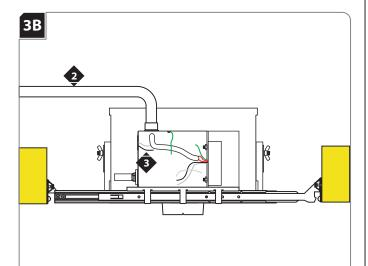
2 Install the conduit to the housing electrical box.
