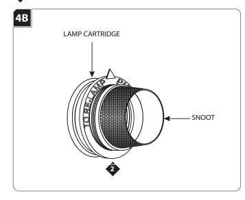
Unscrew the snoot from the lamp cartridge.
