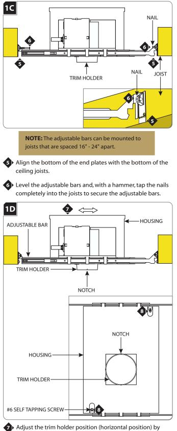
Adjust the trim holder position (horizontal position) sliding the housing on adjustable bars.
