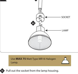
Push the lamp pins completely into the socket holes.
