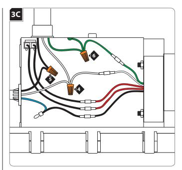
Connect the neutral power line wire to the white transformer wire and the white thermal protector wire with the wire nut.
