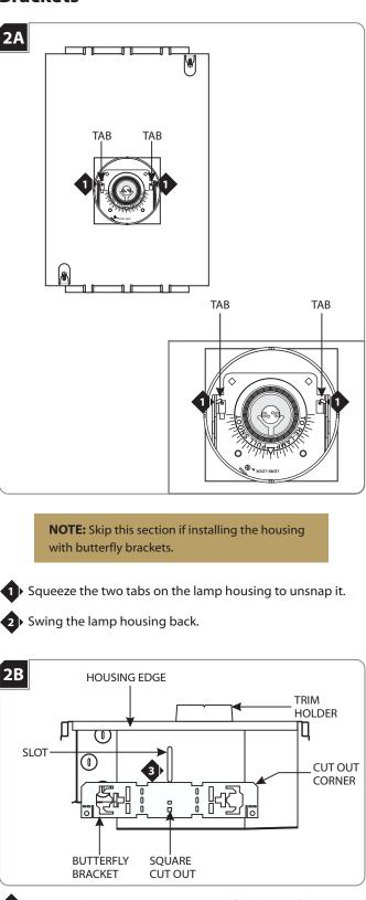
Line up the square cut out section of the butterfly bracket with the housing slot. Make sure the cut out corner of the butterfly bracket is against the housing edge.
