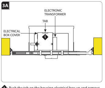
1 Push the tab on the housing electrical box up and remove the electrical box cover.
