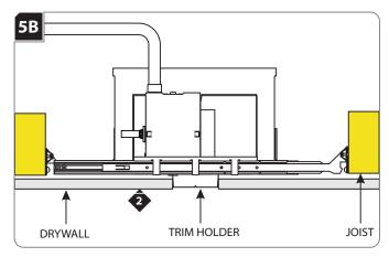
Align the cut out section of drywall with the trim holder and install the drywall.
