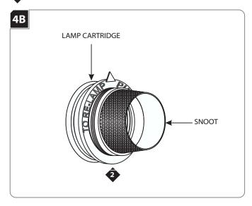
Unscrew the snoot from the lamp cartridge.
