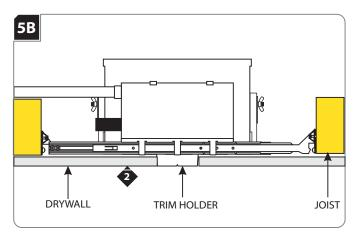
Align the cut out section of drywall with the trim holder and install drywall.
