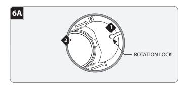
**NOTE:** The lamp housing can rotate 361°. When using a square trim, feel for detents at 90° increments to properly align the lamp to the trim.
