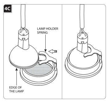
Slide the lamp holder spring completely onto back of the MR16 lamp so that the edge of the lamp snaps into the lamp cartridge assembly.
