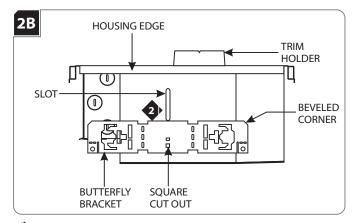
Line up the square cut out section of the butterfly bracket with the housing slot. Make sure the beveled corners of the butterfly bracket are toward the housing edge.
