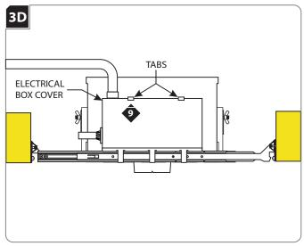
PREPLACE the electrical box cover. Make sure that the top edge of the cover snaps under the tabs.
