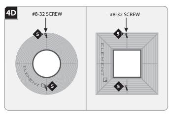
Secure the plaster ring in place with the two provided flat head #8-32 screws. Make sure that the screws penetrate through the drywall into the housing screw holes.
