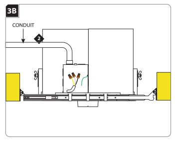
2 Install the conduit to the housing electrical box.
