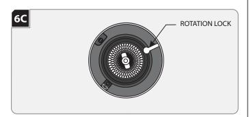
**NOTE:** Lamp housing can rotate 361° horizontally.
