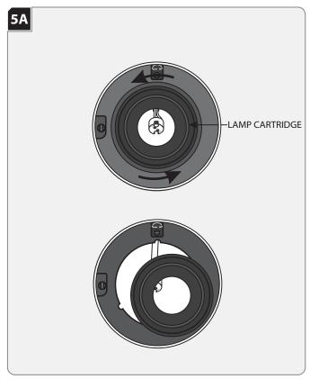
To release the lamp cartridge, rotate it counter clockwise and gently pull out the assembly.
