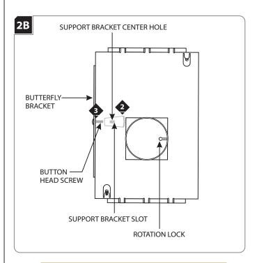
**NOTE:** If necessary, pull the rotation lock down to rotate the lamp housing.
