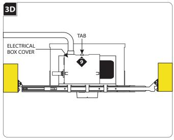
Properties Replace the electrical box cover. Make sure that the top edge of the cover snaps under the tab.
