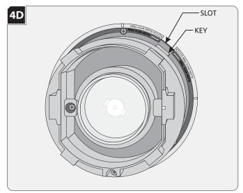
Line up the lamp holder key with the slot in the housing and push the lamp holder in to the housing until the magnets take hold.
