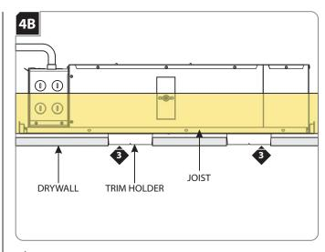
Align the cut out section of drywall with the trim holders and install the drywall.
