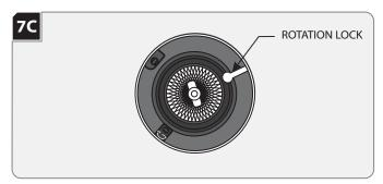
**NOTE:** Lamp housing can rotate 361° horizontally.
