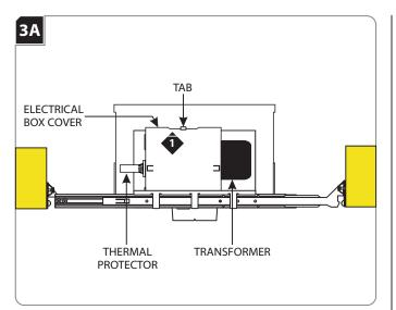
Push the tab on the housing electrical box up and remove the electrical box cover.
