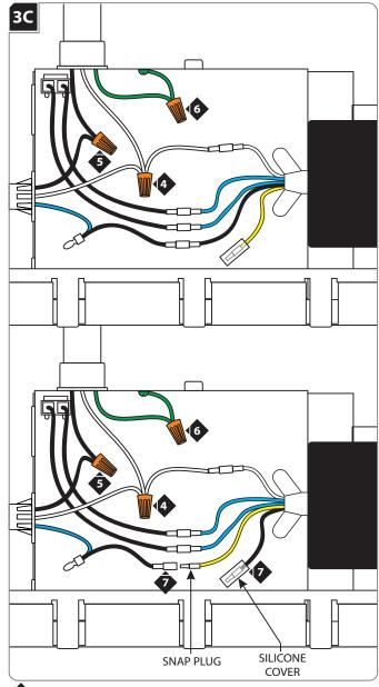
Connect the neutral power line wire to the white transformer wire and the white thermal protector with a wire nut.
