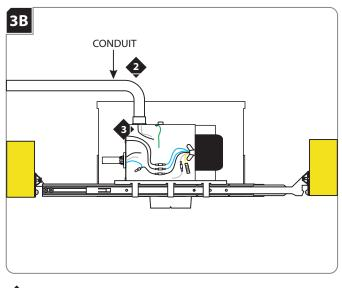
2 Install the conduit to the housing electrical box.
