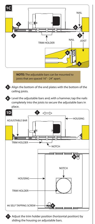
When the desired location is achieved, tighten the two #6 self tapping screws to lock the housing onto the adjustable bars.
