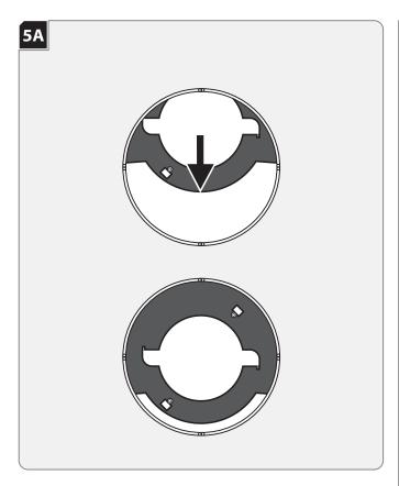
Ensure that the lamp housing is centered to the aperture by pulling it to the center of the housing. When centered the locking pin will be engaged.
