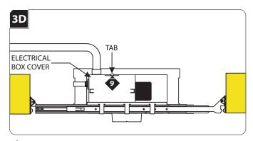
Properties a Replace the electrical box cover. Make sure that the top edge of the cover snaps under the tab.
