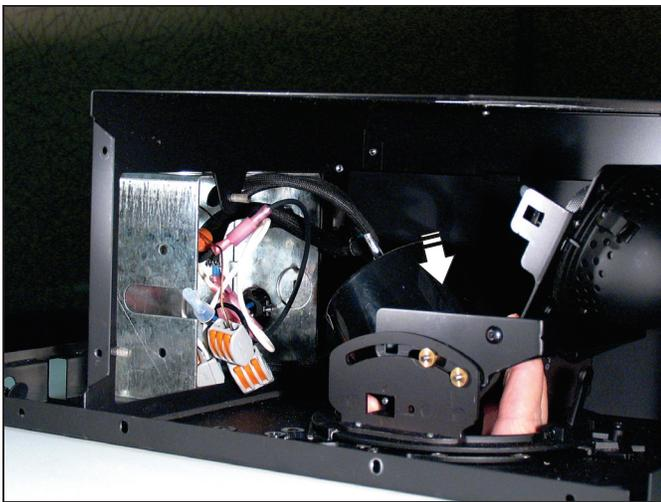
**8** Pull the transformer out of the housing. Do not disconnect any wires at this time. The wires have enough slack to pull the transformer completely out without disconnecting.
