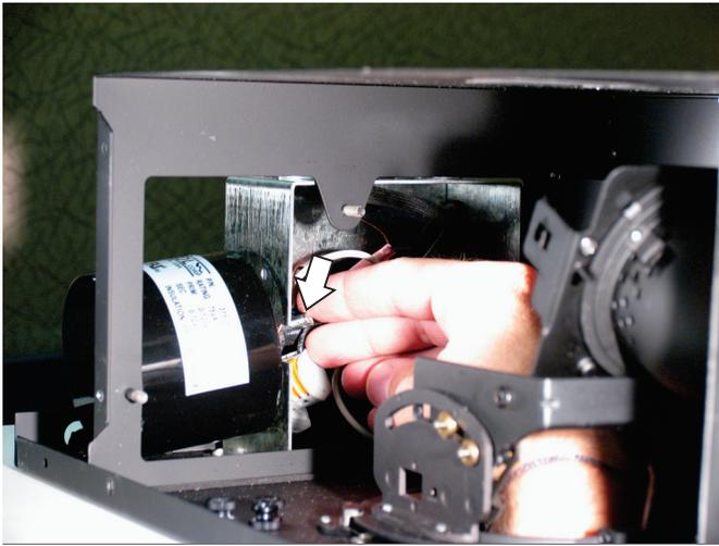
**7** Remove the large wing nut inside the electrical box. This wing nut holds the transformer in place.
