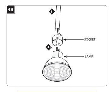
Use MAX 75 Watt Type MR16 Halogen Lamp.
