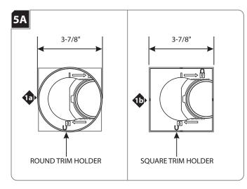
For housings with round trim holder, mark a 3-7/8" diameter circle on drywall. Cut out the marked section.
