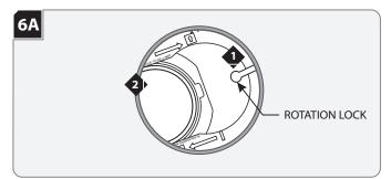
**NOTE:** The lamp housing can rotate 361°. When using a square trim, feel for detents at 90° increments to properly align the lamp to the trim.
