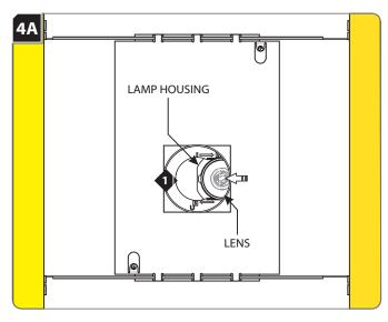
Slide the lamp housing toward the center of the opening. Align the marking on the lamp holder with the "unlocked" symbol.
