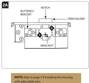
Slightly loosen the wing nut to slide the butterfly bracket up or down.
