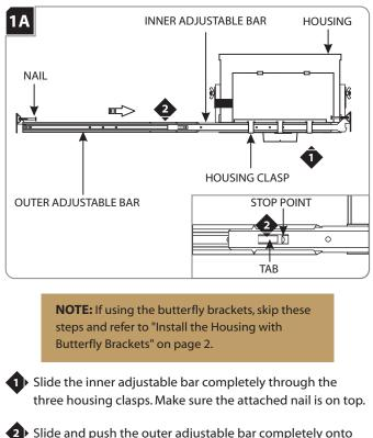
2 Slide and push the outer adjustable bar completely onto the inner adjustable bar so that the tab clicks into place behind the stop point. This will prevent the adjustable bars
