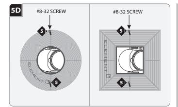
5 Secure the plaster ring in place with the two provided flat head #8-32 screws. Make sure that the screws penetrate through the drywall into the housing screw holes.
