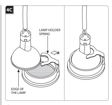
5 Slide the lamp holder spring completely onto back of the MR16 lamp so that the edge of the lamp snaps into the lamp cartridge assembly.
