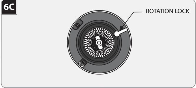
**NOTE:** Lamp housing can rotate 361° horizontally.
