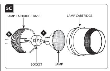
Use **MAX 50** Watt Type MR16 Halogen Lamp.
