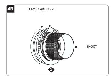
Unscrew the snoot from the lamp cartridge.
