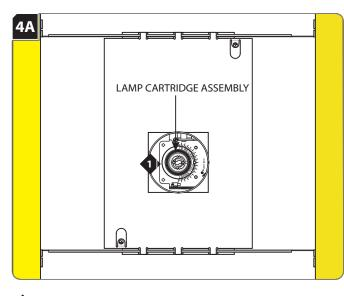
Pull the snoot to remove the lamp cartridge assembly.
