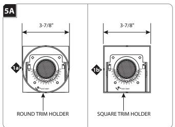
For housings with round trim holder, mark a 3-7/8" diameter circle on drywall. Cut out the marked section.
