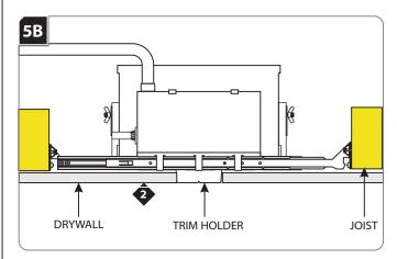
2 Align the cut out section of drywall with the trim holder and install drywall.
