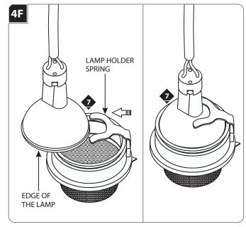
Slide the lamp holder spring completely onto back of the MR16 lamp so that the edge of the lamp snaps into the lamp cartridge assembly.
