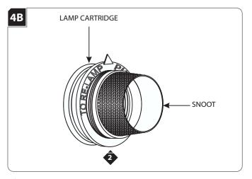
Unscrew the snoot from the lamp cartridge.
