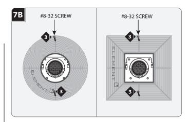
Secure the plaster ring in place with the two provided flat head #8-32 screws. Make sure that the screws penetrate through the drywall into the housing screw holes.
