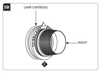
Unscrew the snoot from the lamp cartridge.
