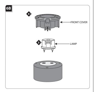
Use **ONLY 18 WATT** proprietary Element Lighting LED lamp.
