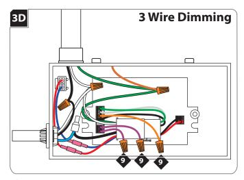
For 3 wire driver applications, properly connect the orange (dimmed hot) and the two purple wires (dimming/digital bus).
