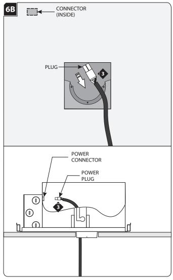
Disconnect the lamp power plug from the connector inside the housing on the electrical box side.
