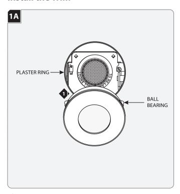
Align the trim ball bearings with the inner edge of the plaster ring.
