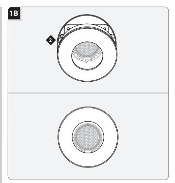
Push the trim into the plaster ring so that the three ball bearings snap into the plaster ring walls.
