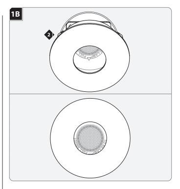
Push the trim into the trim holder so that the three spring connectors snap into the trim holder edge.
