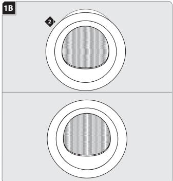
Push the trim into the trim holder so that the spring clips snap into the trim holder.
