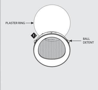
Align the trim ball detents with the inner edge of the plaster ring. Make sure the lamp and trim are pointed in the same direction. There are printed markings on the trim that indicate "TO LIGHTED WALL."
