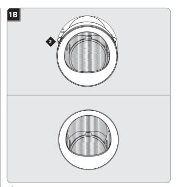
Push the trim into the plaster ring so that the ball detents snap into the plaster ring walls.
