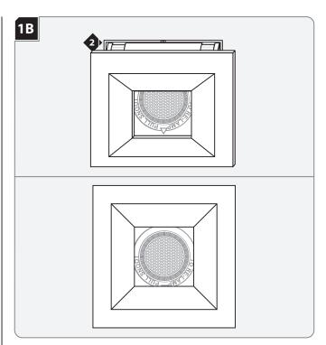
Push the trim into the trim holder so that the four spring connectors snap into the trim holder edge.
