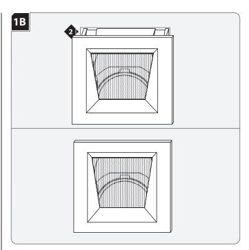
Push the trim into the trim holder so that the spring clips snap into the trim holder edge.
