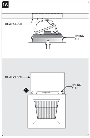
Align the trim spring clips with the inner edge of the housing trim holder. Make sure the lamp and trim are pointed in the same direction. There are printed markings on the trim that indicate "TO LIGHTED WALL."
