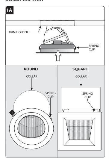
Align the trim spring clips with the inner edge of the housing collar. Make sure the lamp and trim are pointed in the same direction. There are printed markings on the trim that indicate "TO LIGHTED WALL."
