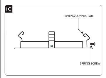
Install the large spring connectors and secure them by reinstalling the spring screws.
