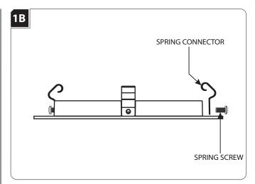
Replace the pre-installed spring connectors by removing the spring screws.
