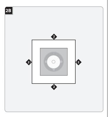
Gently push the trim into the housing so that the four spring connectors snap into place.
