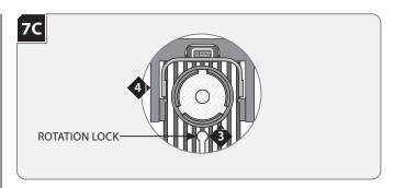
**NOTE:** Lamp housing can rotate 361° horizontally.
