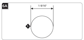
Use a 1-9/16" hole saw to cut out the ceiling or wall where the test switch will be installed.
