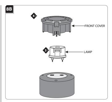
Use **ONLY 18 WATT** proprietary Element Lighting LED lamp.
