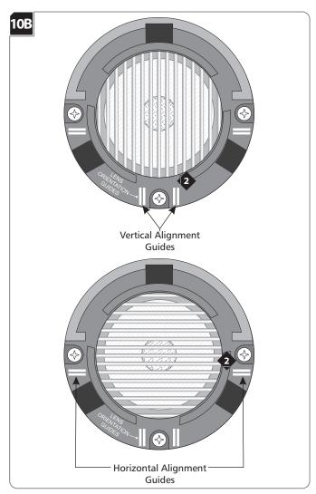
Use the lens orientation guides to align linear spread lenses vertically or horizontally.
