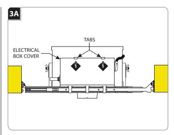
Push up on the tabs on the electrical box and remove the electrical box cover.
