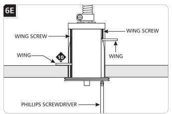
Tighten the two phillips screws (an electric screwdriver will help) until the wings secure the test switch port into the hole.
