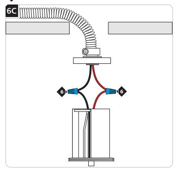
Connect the red and black wires in the test switch port to the same color wire in the flexible conduit using wire nuts.
