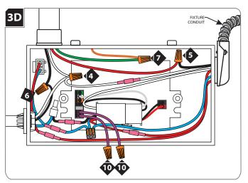
**EcoSystem Fade-to-Black** applications, properly connect the two purple wires (dimming/digital bus).
