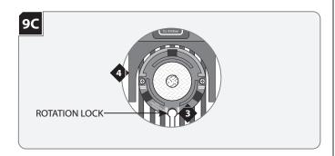
**NOTE:** Lamp housing can rotate 361° horizontally.
