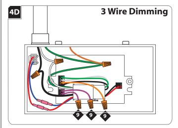
Pror 3 wire driver applications, properly connect the orange (dimmed hot) and the two purple wires (dimming/digital bus).
