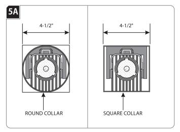
For round trims, mark a 4-1/2" diameter circle on drywall. Cut out the marked section.
