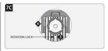
**NOTE:** Lamp housing can rotate 361° horizontally.
