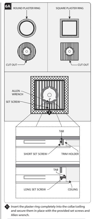
**NOTE**:Longer set screws have been provided for instances where the plaster ring does not reach the collar and must be secured to the inside of the ceiling cutout. Use the short set screws if the trim is installed in the collar.
