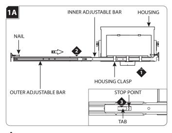
1 Slide the inner adjustable bar completely through the three housing clasps. Make sure the nail is on top.
