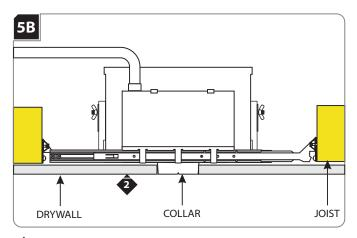
Align the cut out section of drywall with the collar and install drywall.
