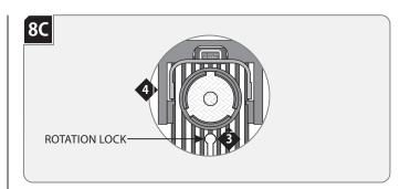
**NOTE:** Lamp housing can rotate 361° horizontally.
