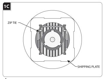
Carefully cut and remove the zip ties to remove the shipping plate.
